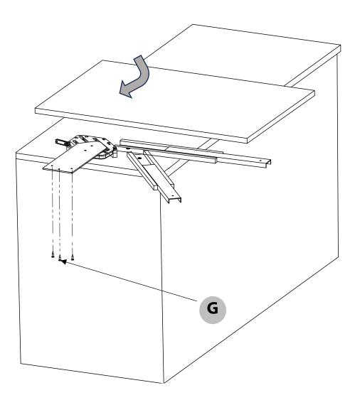
Make sure the moving plate of the mechanism is pointing outwards as shown in the image. Take the upper board and hook the locking plate into the v-shape of the moving plate of the mechanism, fix the 3 screws of the moving plate.
