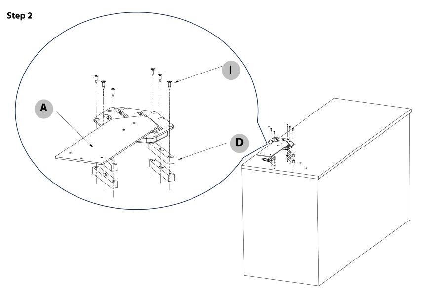
In order to reach all screw holes, move the upper moving plate of the mechanism back and forth.
