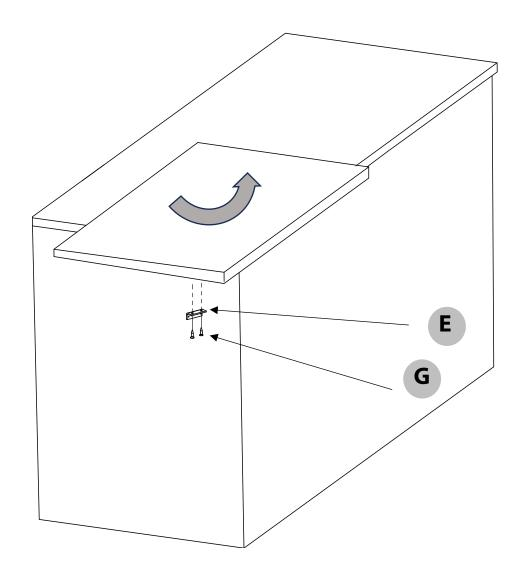
Rotate the upper board by 90 degrees to the right, install the metal angle and your Roto is ready for usage.
