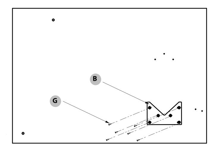
Make sure the moving plate of the mechanism is pointing outwards as shown in the image. Take the upper board and hook the locking plate into the v-shape of the moving plate of the mechanism, fix the 3 screws of the moving plate.
