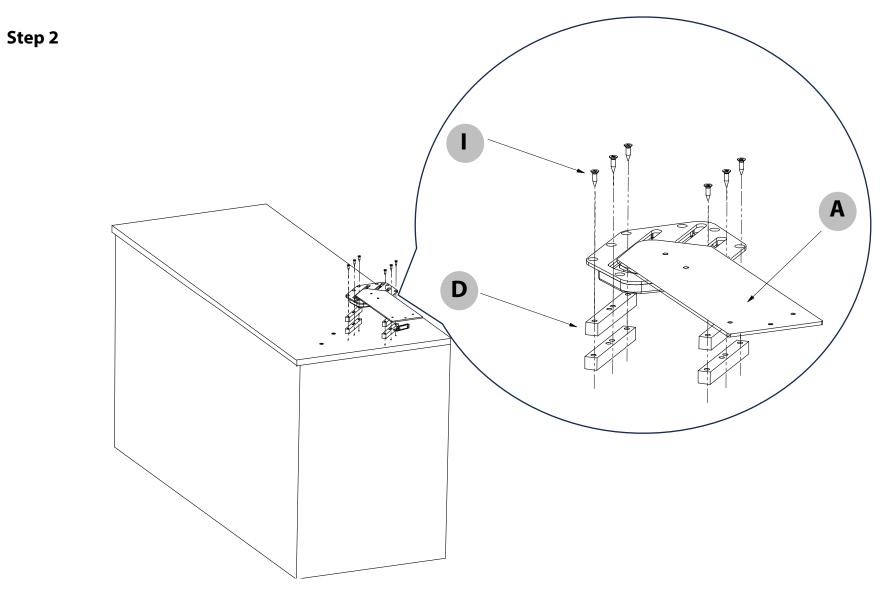
In order to reach all screw holes, move the upper moving plate of the mechanism back and forth.
